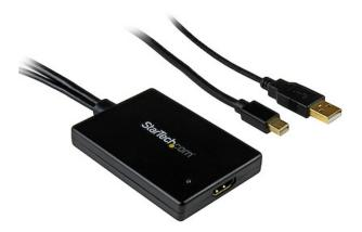
The MDP2HDMIUSBA Mini DisplayPort with USB Audio to HDMI Adapter offers a cost-effective HDMI with audio to Mini DisplayPort link, letting you connect an HDMI-capable HDTV to a device with a Mini DisplayPort output, while saving the expense of upgrading the TV for compatibility. The Mini DisplayPort adapter is the perfect accessory for any of your Microsoft Surface Pro devices with mDP.
